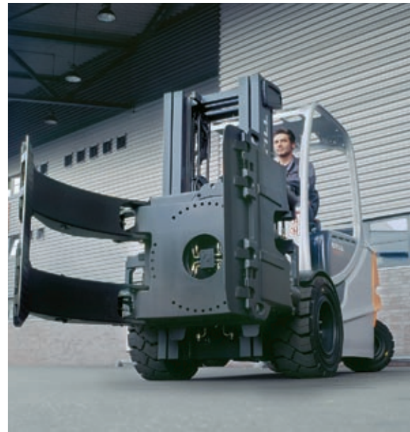
Attachments such as those for handling paper rolls are the applications for INA slewing rings
