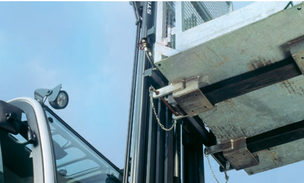
Lift mast and chain guide rollers ensure precise movement of the lifting load
