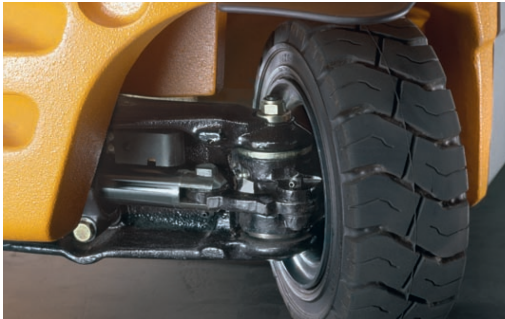
Tie rod: Maintenance-free solutions are also possible here
