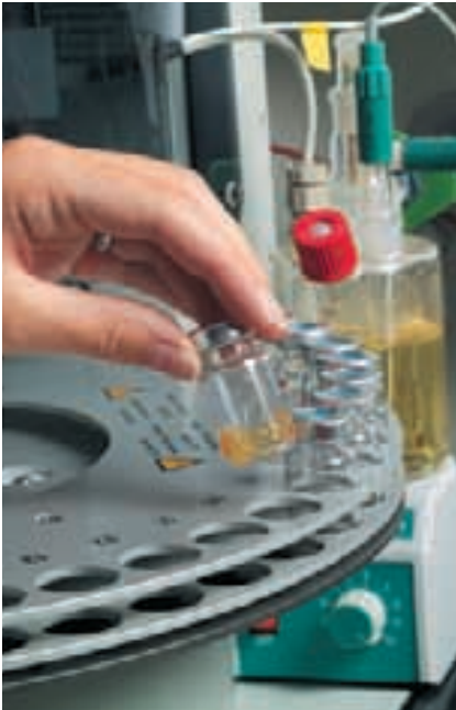
Testing in our in-house lab: Analysis of lubricants for water content
