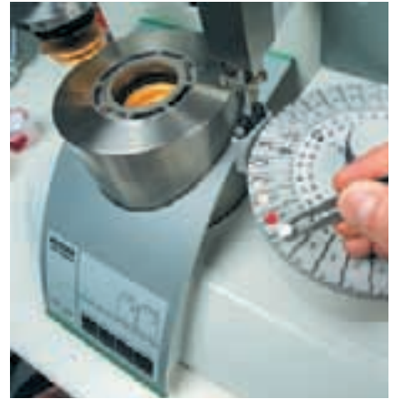
DSC analysis: Temperature behavior of lubricants, analyzed using the latest methods
