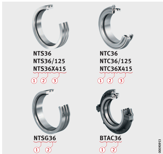
Figure 17 Designation structure of standard seals, examples
